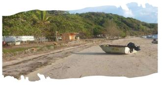
• The study shows an overall erosion trend along the town beach south of Raehome Point with some minor accretion at the southern end, indicating an overall loss of sand under the influence of easterly waves and tidal currents and the presence of the seawall.
